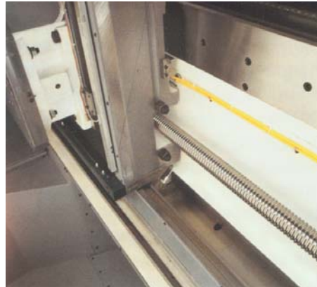
Frictionless hydrostatic ways enhance stiffness and repeatability.
